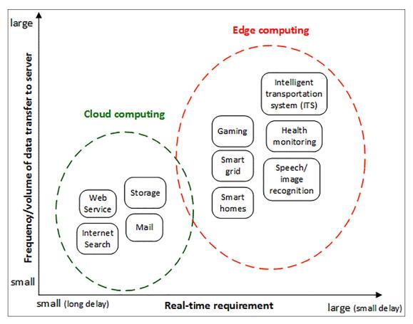
Figure 2 – Cloud Computing versus Edge Computing application areas.
