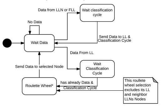
Figure 20 – State diagram for LLN nodes.
