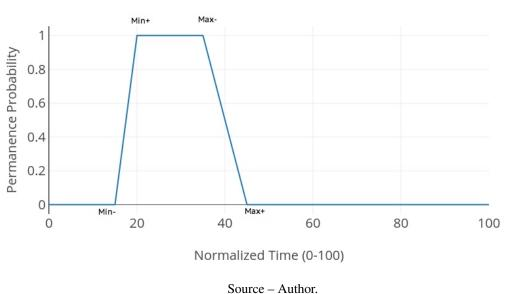
Figure 23 – Trapezoidal temporal model function of device availability.
